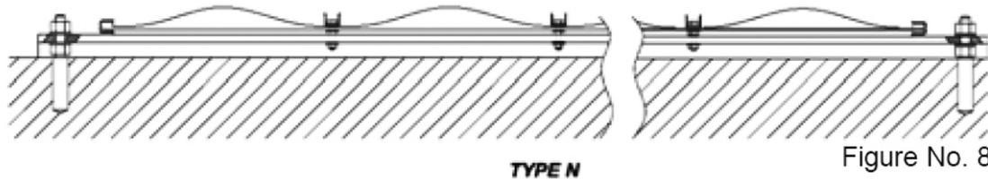
The overall dimensions of this product (Model N 4) are 41” x 158” (104 cm x 400 cm). The clamping system uses a structural perimeter frame with intermediate cross supports as shown in Figure No. 8. The mechanical forces on the structural frame may be estimated as follows:
